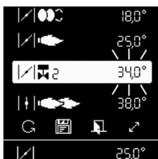
When the flame is detected and has stabilised, the burner switches to stage 1, at the end of the safety time.
